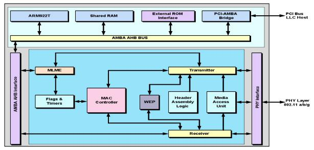
SI24WLAN11 MAC based on SoC design, supports ARM922T processor for management level functionality to address the needs of complex design system, low power consumption and high performance. A shared RAM shall be used for the management operations done by the ARM processor. The AMBA AHB architecture is used for transferring management operations to the ARM processor and the data to the Host layer through PCI-AMBA Bridge.
