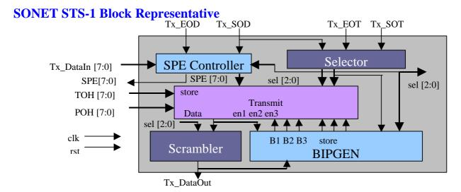
BIPGEN: This module is responsible for the generation of Bit Interleaved parity bits for the section, Line and path overhead.
