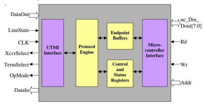
The USB function core consists of five main modules: UTMI Interface, Protocol Layer (PL), Endpoint Buffers, Control and Status Registers (CSRs) and Microcontroller Interface.
